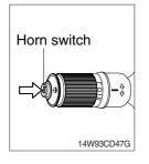
① This switch is at the end of left side multifunction switch. On pressing, the horn sounds.
